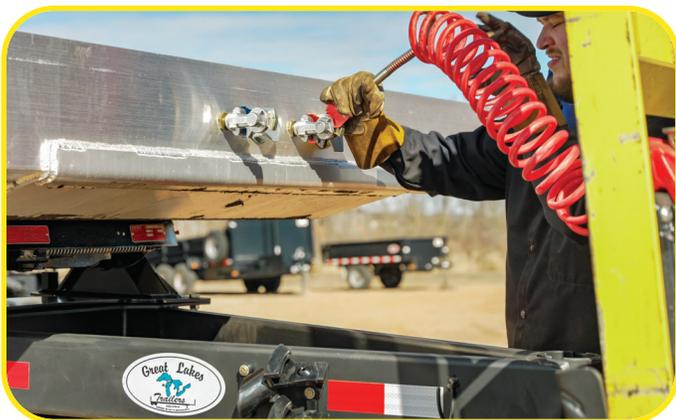
Air reservoirs with airline and glad hand connection to release trailer air brake system
