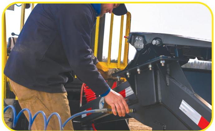
Air reservoirs can be refilled from shop air with standard air tool coupling
