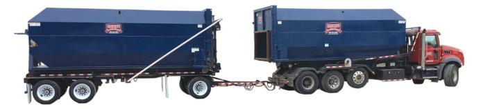
Trucks with cable or hook lift systems can easily transfer containers on and offthe rear of the trailer in minutes!
