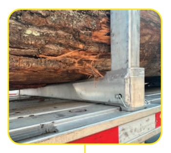
**Alum-A-Log** bunk Pin securement system, crossbar pins under trailer stake pockets, the aluminum uprights pin into the crossbar.
