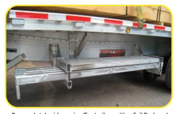
Dropped style side carrier (For trailers with a Coil Package)
