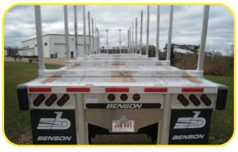
3 piece bunk consisting of 1 aluminum crossbar and 2 aluminum uprights. Crossbars can be used as dunnage when uprights are removed for transporting other products such as lumber.
