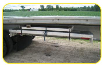
Standard side carrier – Gain the ability to stow your **Alum-A-Log Bunk Systems** under the trailer bed when not needed to make room for standard freight.
