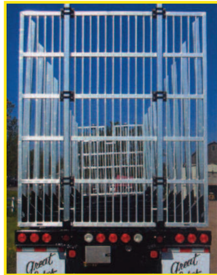
Patented All Aluminum Headboards and Adjustable Bolt-On Bracket Carrier with Wear Pads.
